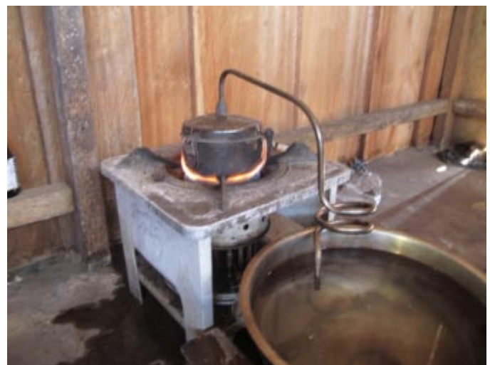
Small-scale technology reduces the impact of mercury which is used in the gold smelting process. A stainless-steel retort captures 99% of the mercury.
