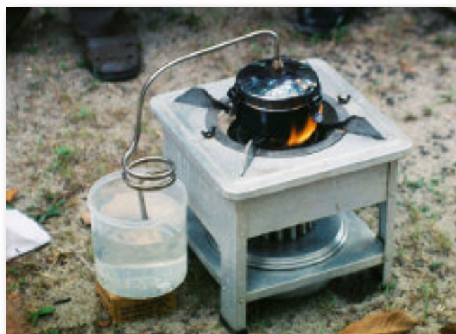
Retorts are popular with miners as they can recycle their mercury.
